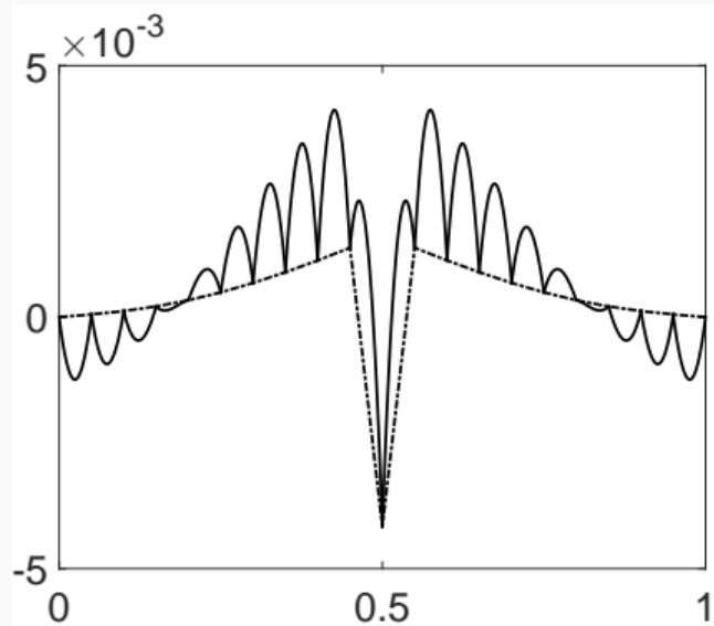
Left: discretization error  $u - u_h$ . Right: algebraic error  $u_h - u_h^9$  (dashed-dotted line) and total error  $u - u_h^9$  (solid line).
