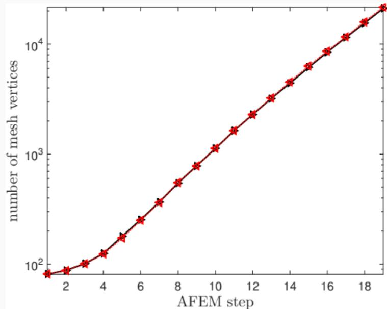
Left: the decrease of the discretization error norm in adaptive FEM that is based on  $EST(u_h)$  (black) and  $EST(u_h^i)$  (red), respectively. Right: the corresponding number of degrees of freedom in refinement steps.
